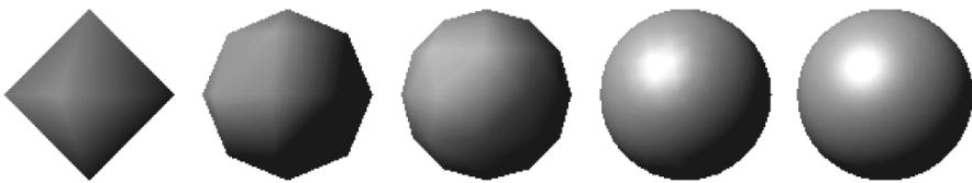
Figure 6.12 Representation of a sphere with different tessellations
