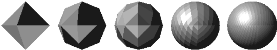
Figure 8.10 A sphere in different tessellations rendered with flat shading
