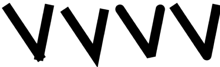
Figure 3.24 Different line endings and joins
